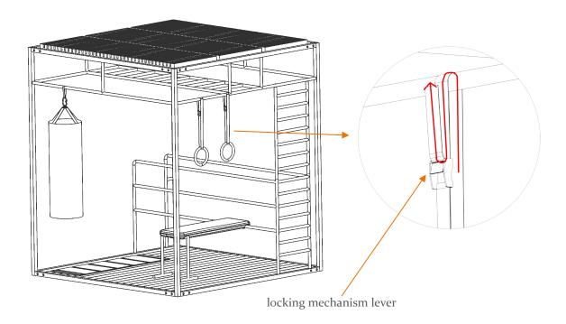
To attach the rings, simply slide the band over the bar and then pass it through the locking mechanism. To adjust the height of the rings, press the lever on the mechanism and slide the band until it reaches the desired position.
